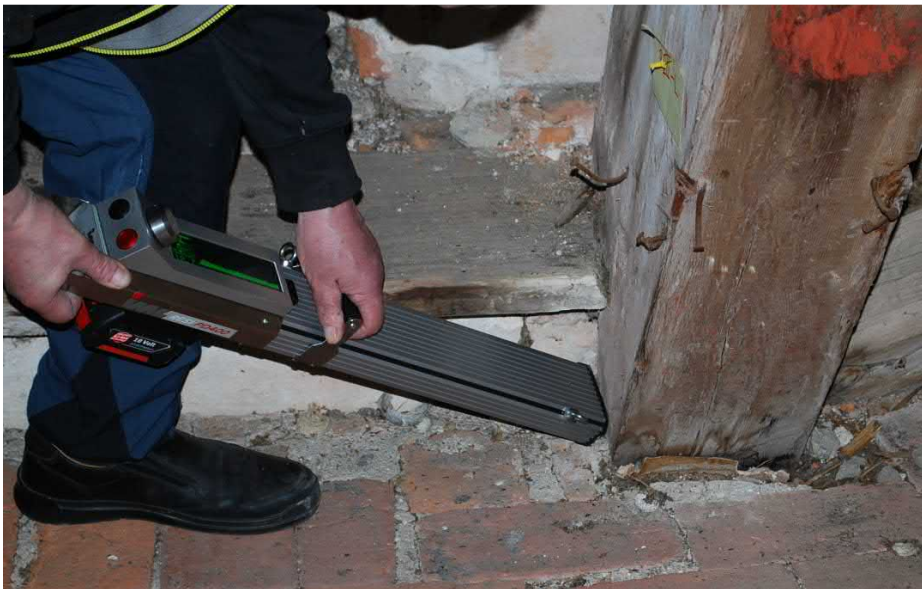
Figure 40. Resistance drilling performed to the post of the leaning trestle (PIIII) on the southwest side of the roof. The figure also shows that birch bark has been used to protect the embedded parts of the post from moisture.
