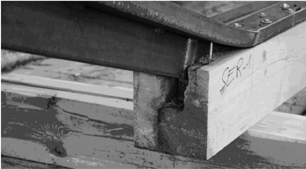
Figure 14. Failure occurred in steel profile during the bending test [48, p. 44].
