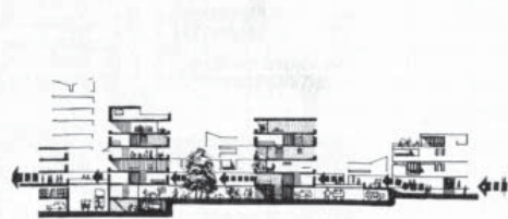
1040, 1041, 1042, 1043 Hook new town: network of roads and of pedestrian ways; plan of civic centre, with separation of pedestrian and motor traffic; cross section through a residential area (from the London County Council book, 1961)
